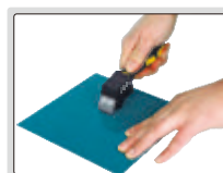
step 1: make grid cutting on surface
