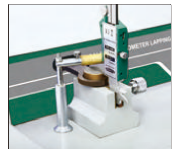
lapping measuring surfaces of caliper lower jaws
