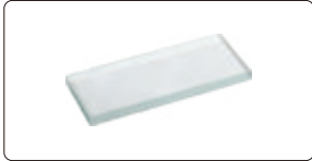
50mm reading scale (check magnification accuracy)
