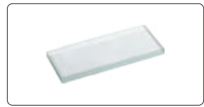
50mm reading scale (check magnification accuracy)
