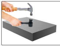
hammer impact to apply test force
