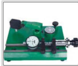
inspect accuracy of dial indicators (range 0-25mm)
